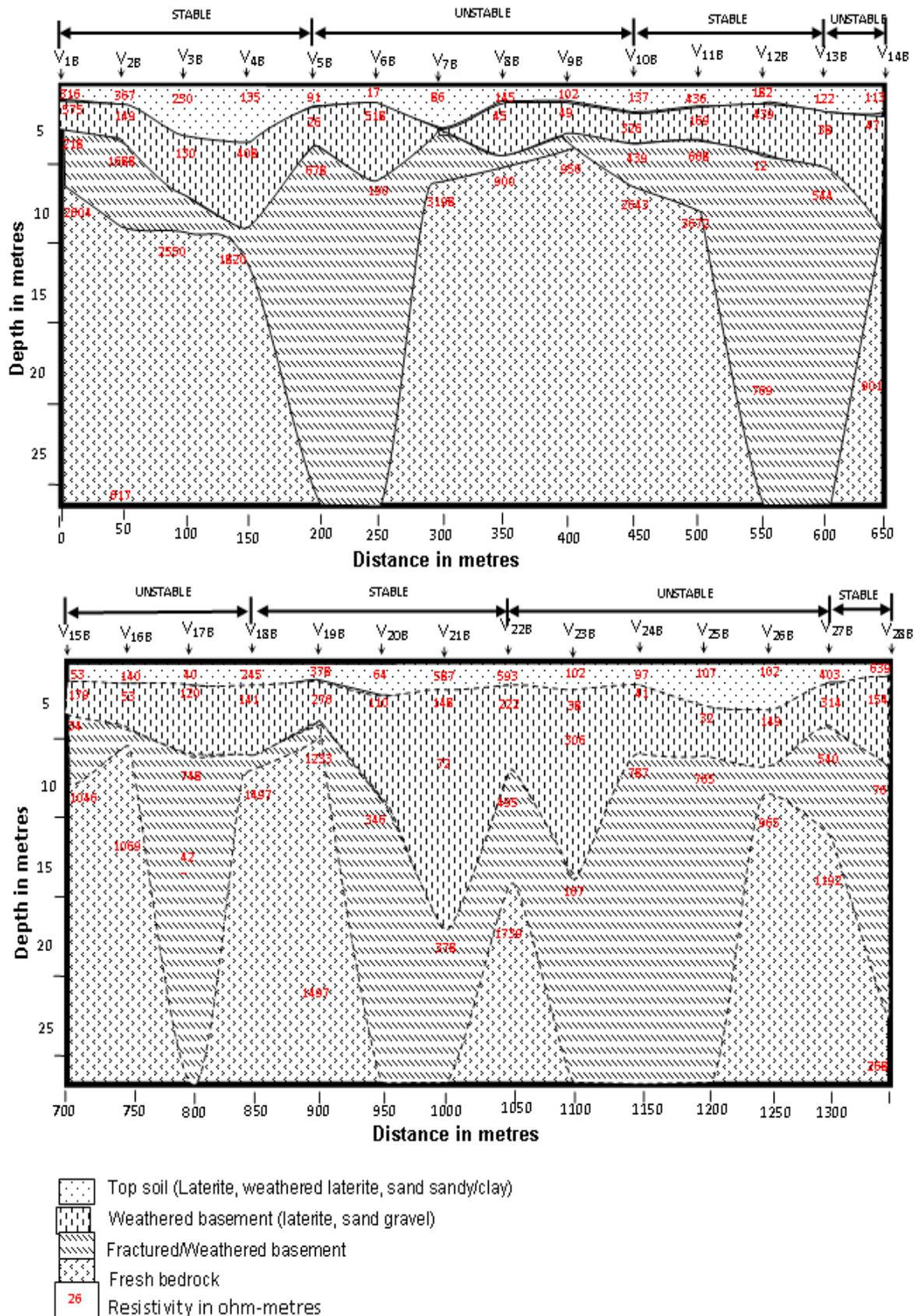
Figure 5: Geoelectric and Geologic Sections Along Profile P<sub>2</sub>
