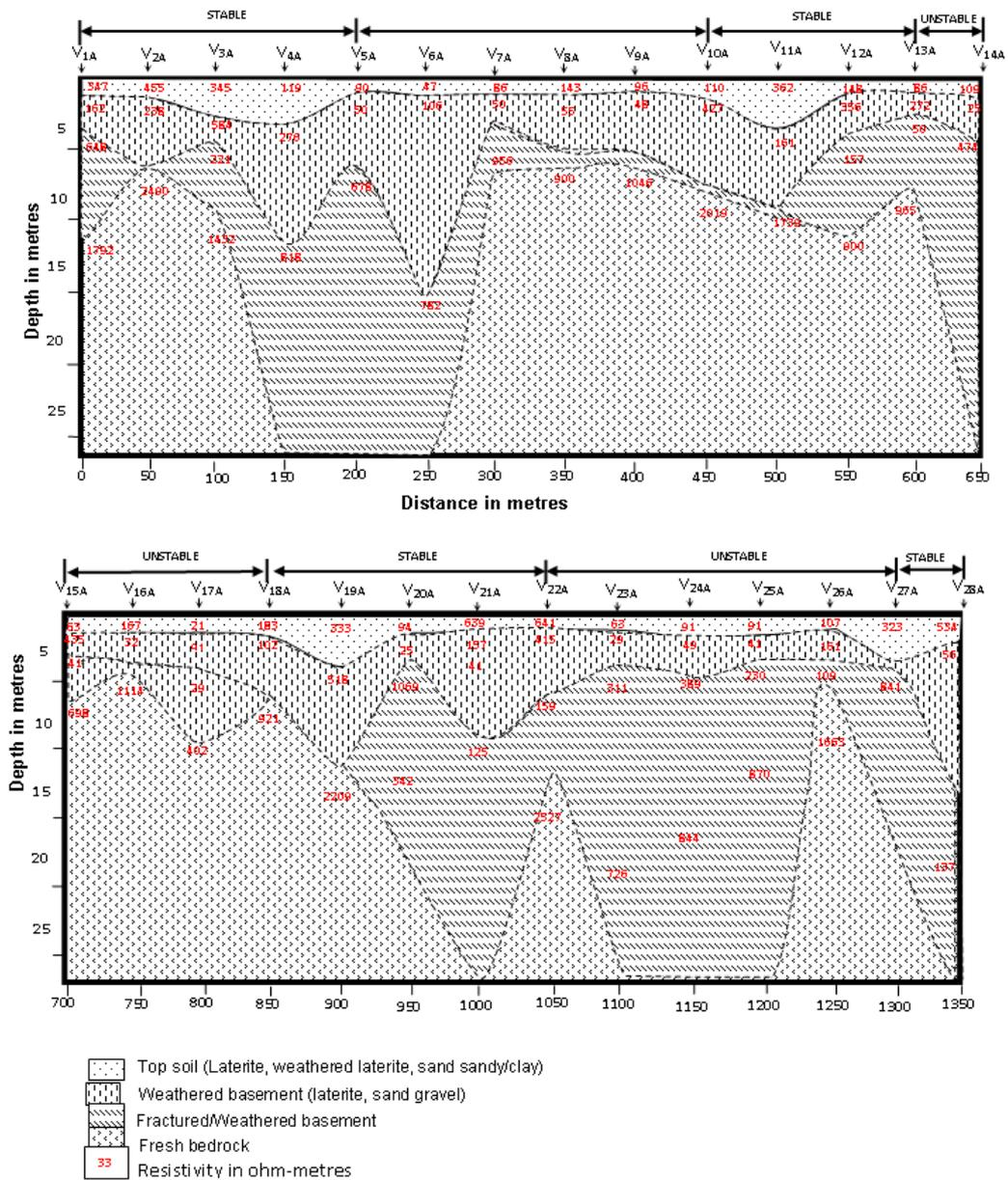
Figure 4: Geoelectric and Geologic Sections Along Profile P<sub>1</sub>
